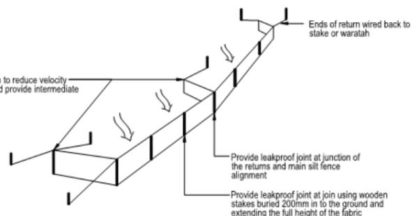
Silt fence with returns and support wire
