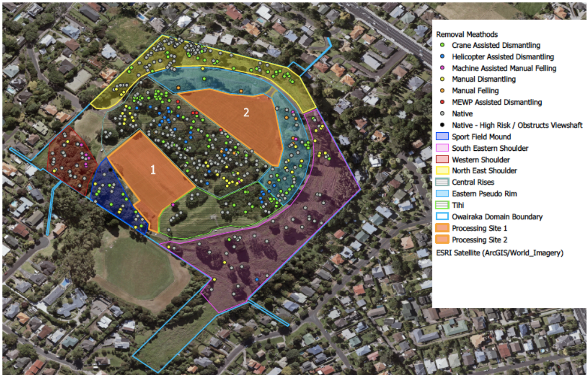
Figure 3 – Aerial map showing the operating zones, tree locations and removal methods
