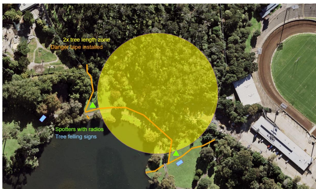
Figure 3: Western Springs Park Public Protection Zone. Public to be excluded when trees are felled within area denoted by green circle.
