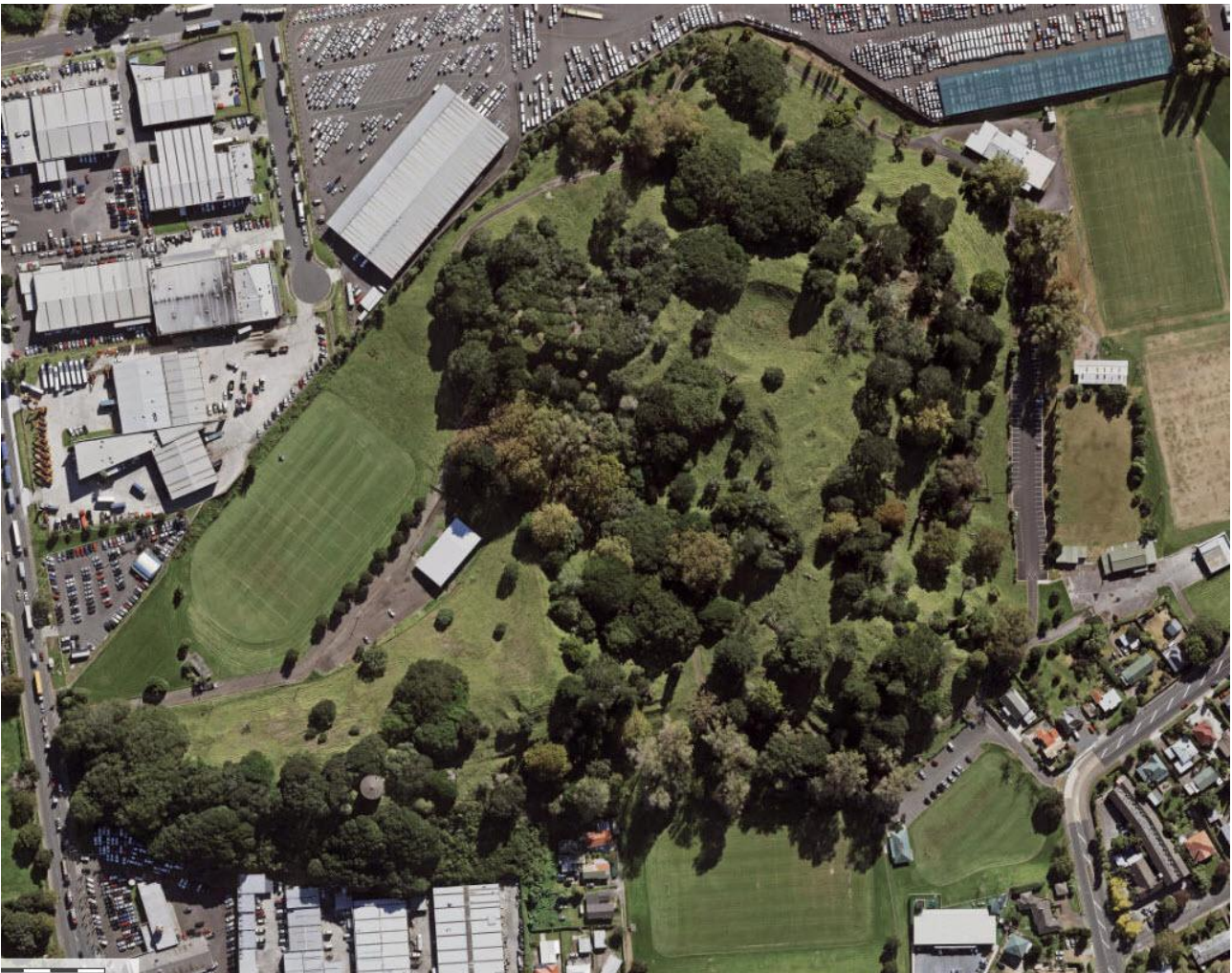
Figure 10. 2017 aerial photograph, this shows that most of the quarry off Great South Road is still in operation and has been extended somewhat, the slopes upto the tihi have been rehabilitated and sloped prior to becoming part of the Reserve. Features between the Domain and Portage Road have been removed (compare to Figures 8 and 9).
